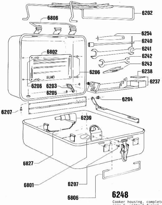
Cooker housing, complete, as shown on page 6, without funnel, chain, grate, accessories and spare parts.
