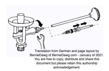
3.3 REPLACING THE REGULATING SPINDLE
